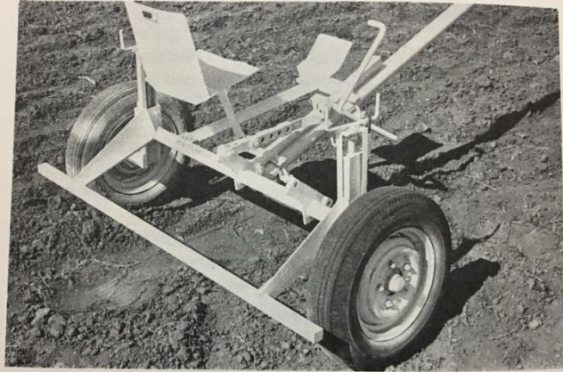
The Nikart is a newer model of the wheeled tool carrier, designed by the National Institute of Agricultural Engineering, UK, in collaboration with ICRISAT.
